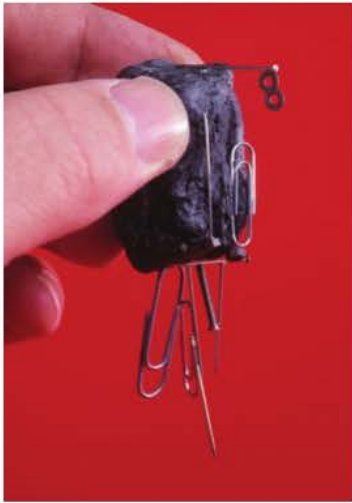
▲ Not all magnets are human-made; some rocks (for example, this piece of magnetite) are naturally magnetic.
