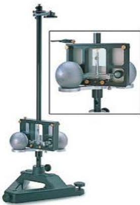
The modern equivalent of the apparatus used by Cavendish to measure G in 1798.
