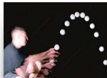
▲ A stroboscopic photograph of a projected ball.
