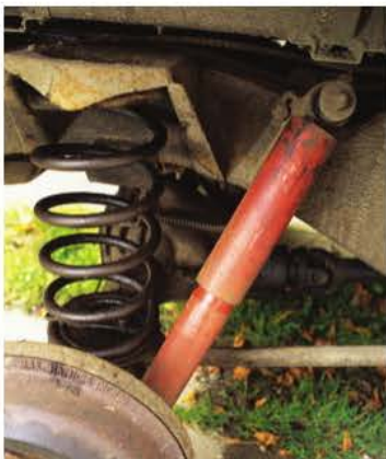
A car suspension is critically damped to prevent the car oscillating after it goes over a bump in the road.
